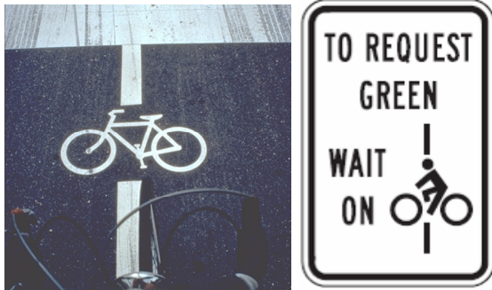
Figure 2.10. Signal activation marking and sign.
